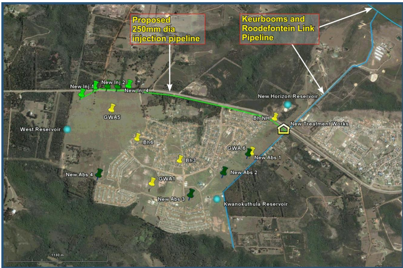
FIGURE 3.12 INFRASTRUCTURE COMPONENTS FOR OPTION 2 – RECHARGING WITH KEURBOOMS RIVER WATER AND TREATING IN NEW TREATMENT WORKS (GOOGLE EARTH, 2010)
