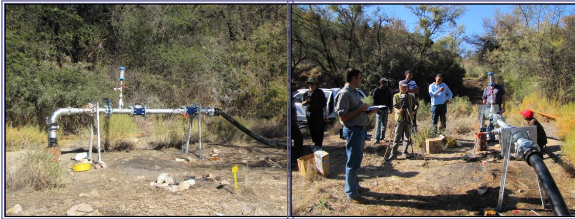
PHOTO 1 & 2: THE BOREHOLE INJECTION RIG USED FOR THE PRINCE ALBERT ARTIFICIAL RECHARGE TESTS
