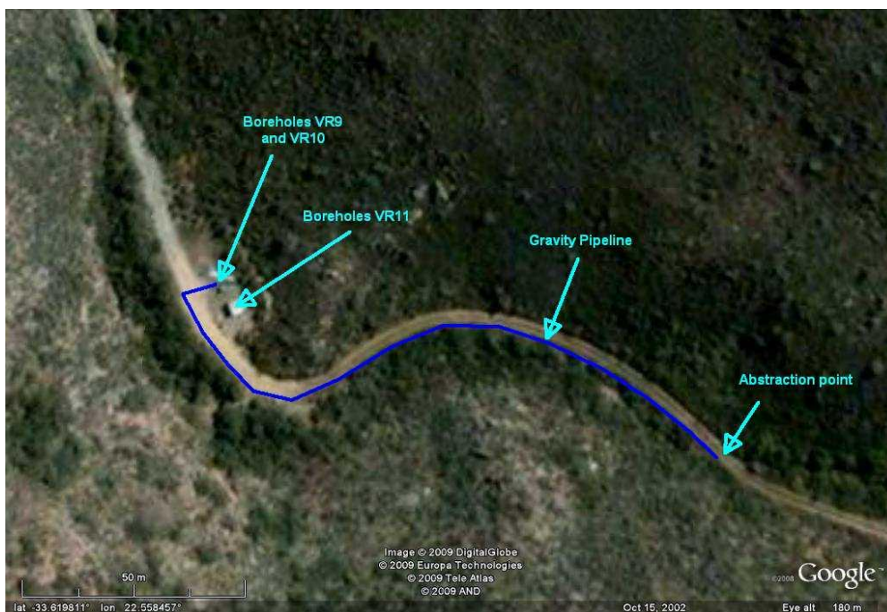
FIGURE 7.2 THE PROPOSED INFRASTRUCTURE TO TEST AR IN THE UPPER-MOST PART OF THE VERMAAKS RIVER WELLFIELD (GOOGLE EARTH, 2010)
